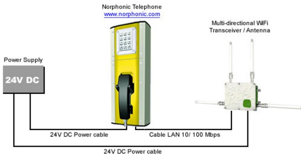
The flexibility of the Norphonic VoIP Mining Telephones therefore means that it could be used on a fixed fiber cable layout or in a wireless VoIP environment. There are no particular barriers to installing Wireless / WiFi solutions, but the network designer should be aware of potential voice quality pit-falls and plan for these. Some key things to be aware of in terms of voice quality when designing your network layout:
